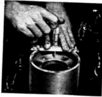
Measuring the depth of a shoulder with the Starrett No. 445C-3RL Micrometer Depth Gage.
